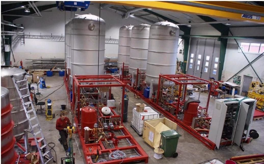
Picture from Ageratec's workshop; two units of PE24000 Biodiesel Processor under production.
