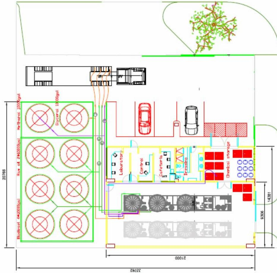
One example of layout for the PE240000 Biodiesel processor which leaves the possibility to scale up
